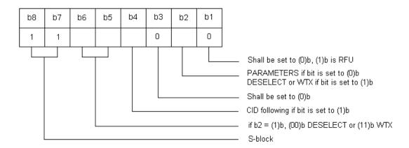
Figure 17 — Coding of S-block PCB
